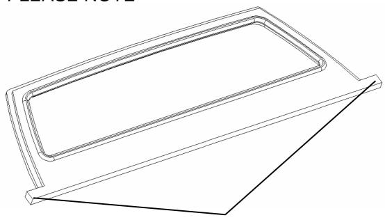
These tabs need to be trimmed approximately 1.5mm at each end before fitting to the front cab.
