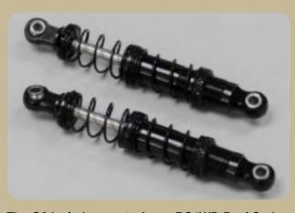
The G2 includes a set of new RC4WD Dual Spring Shocks. An all new design, this ultimate scale shock has realistic looks and the ultimate in performance. Machined from billet aluminum with dual springs and totally rebuildable.
